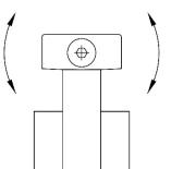
Never allow pads to span straight and back tapered sections at the same time. This will result in damage to the workpiece, tooling and the Grinding AUTO REST®
